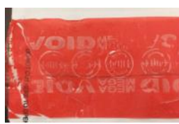
Attempt to open tape after cold freeze attacked
