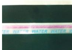
Result of being exposed to conditions above 60°C or being attacked by heat elements with temperatures above 60°C
